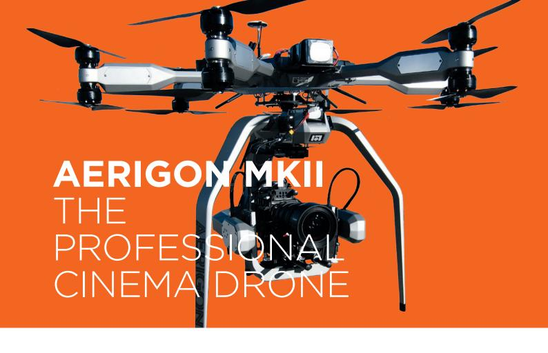
THE AERIGON BY INTUITIVE AERIAL is an elite cinema drone system for professional cinematographers and broadcast specialists. The AERIGON's proprietary power distribution system and dual coaxial design with 12 powerful counter-rotating rotors and pre-preg carbon-fiber exoskeleton provides the power, precision and stability to carry the weight of sophisticated camera configurations with pro zoom lenses and full FIZ (Focus, Iris & Zoom) control.
